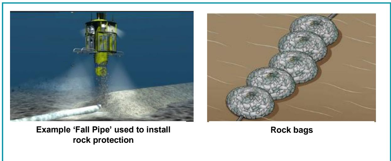
Plate 5.6 Example 'Fall Pipe' used to install rock protection
