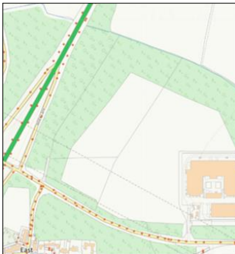
Figure 3-3: Highway drainage system and gully's locations within Brock Lane
