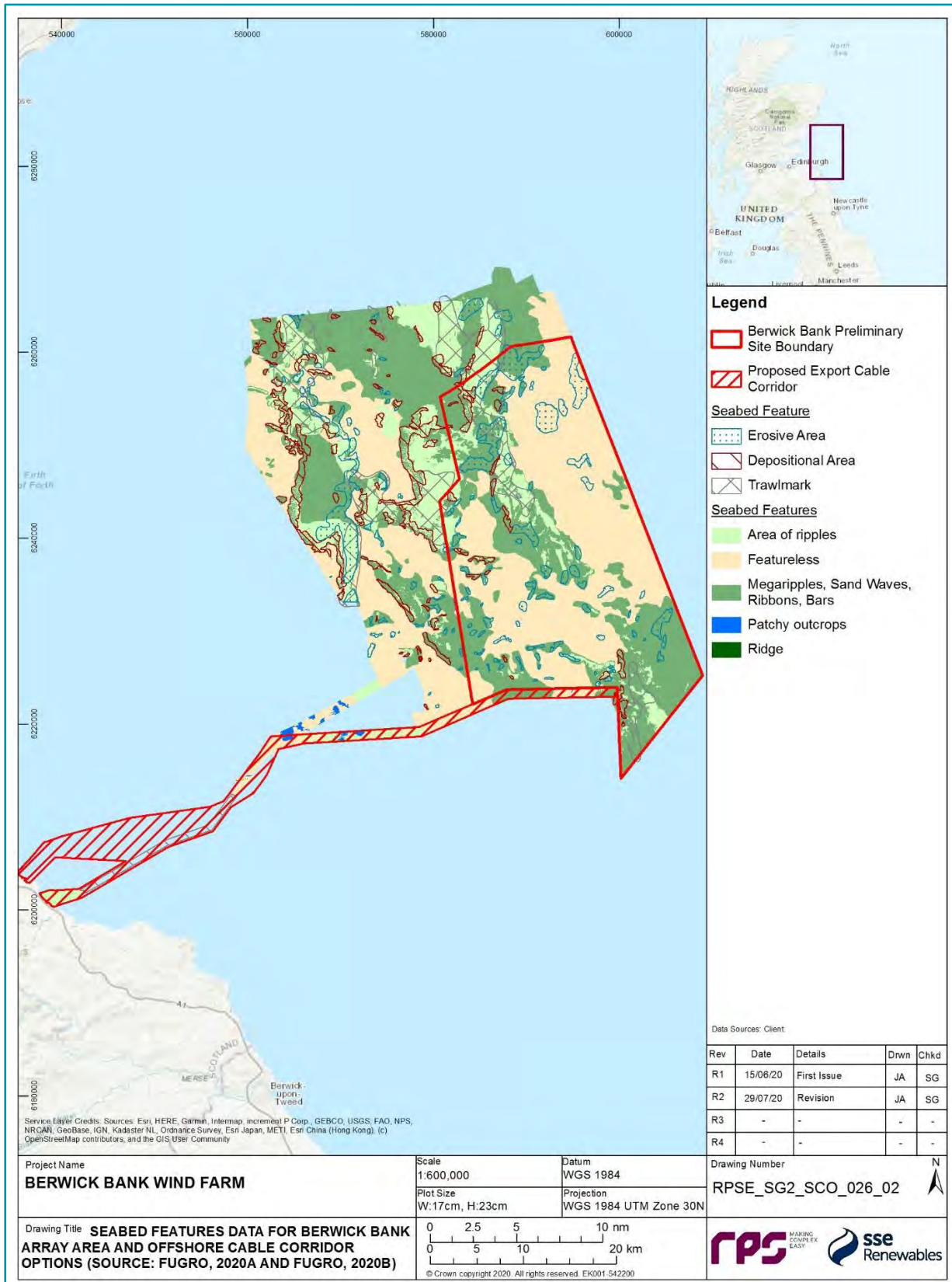
Figure 7.5: Seabed Features Data for Array Area and Proposed Export Cable Corridor (Source: Fugro, 2020a and Fugro 2020b).
